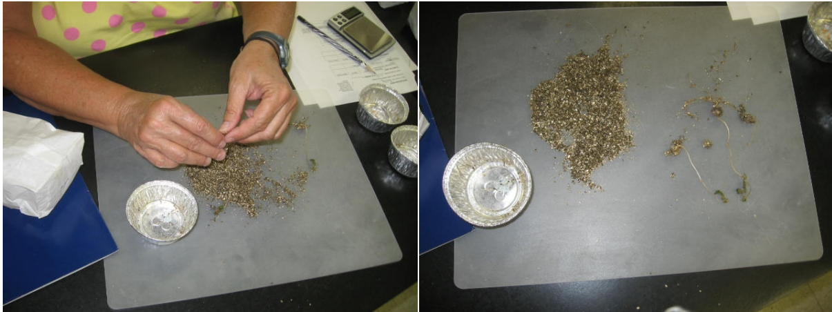
Fig. 3. Separating the plant biomass from the growing medium (vermiculite), using a flexible plastic cutting board as a work surface.
