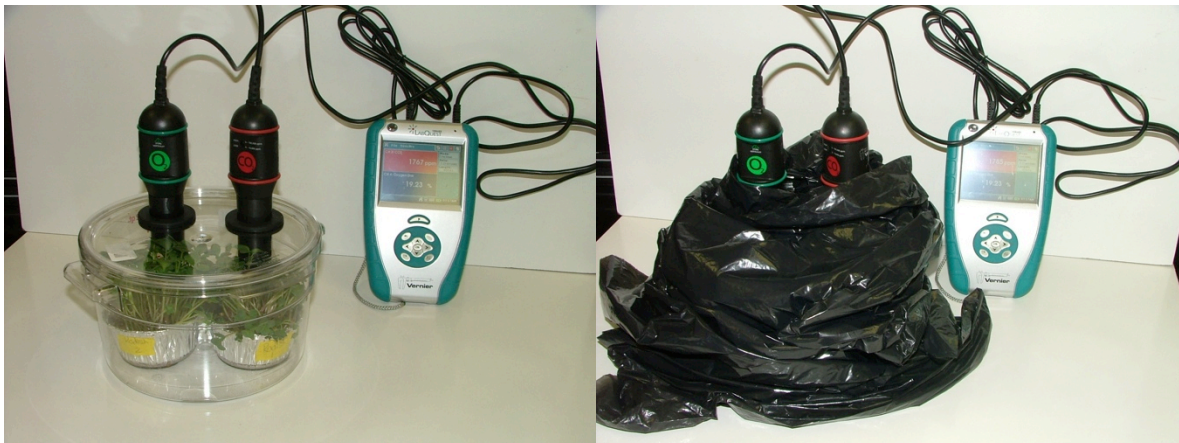
Fig. 2. Illustrating measurement of \text{CO}_2 and \text{O}_2 (optional) concentrations in both light and dark conditions. These measurements were taken in a 2000-mL biochamber available from Vernier Instruments, but could be taken in any reasonably airtight container large enough to hold a number of photosynthesizing plants.
